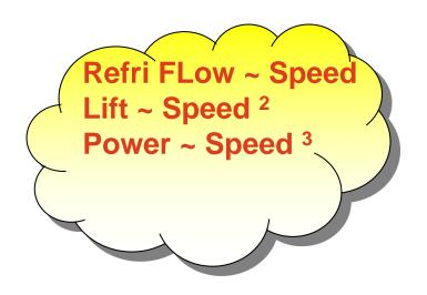
A balance between the speed reduction and vane throttling is needed for 'Surge-Free' Operation at Low Load conditions.
