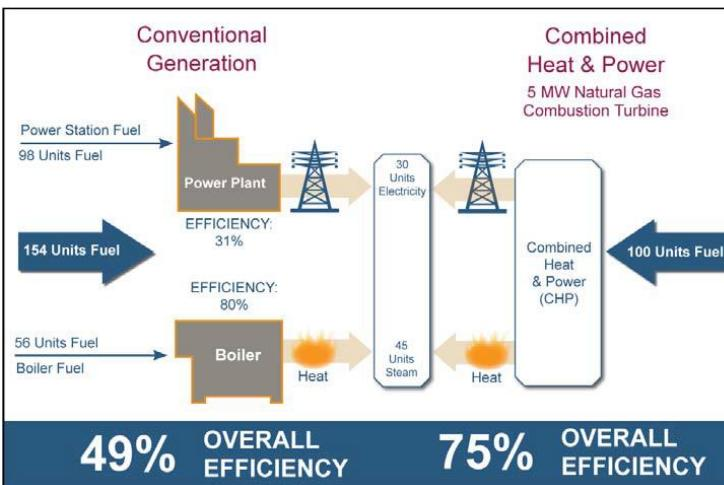
Figure 2: Equivalent Separate Heat and Power Efficiency
