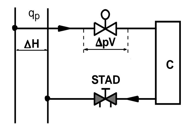
$3 = \frac{\Delta P_{\text{Control valve fullyopen and designflow}}}{\Delta P_{\text{Control valve fullyshut}}}$
