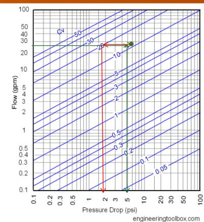
Flow to a FCU of 29 gpm,  $\Delta p$  5 psi and 2 psi in connecting pipes. the commercially available control valves create a design  $\Delta pV$
