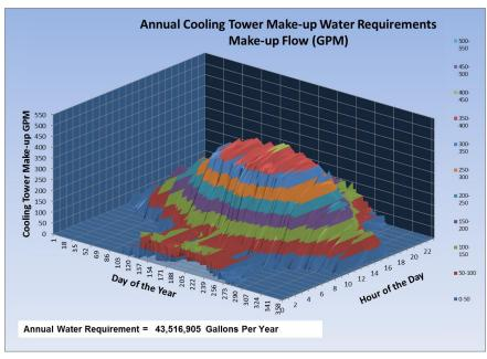
Cooling Tower Only System Annual Water Use = 378,006 m<sup>3</sup> TCHS System 56% Savings
