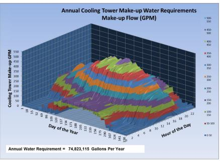
Cooling Tower Only System Annual Water Use = 378,006 m<sup>3</sup> TCHS System 25% Savings
