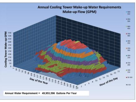
Cooling Tower Only System Annual Water Use = 378,006 m<sup>3</sup> TCHS System 50% Savings
