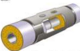
Figure 1: Illustration of the structure of a bonded pipe and a casing joint
