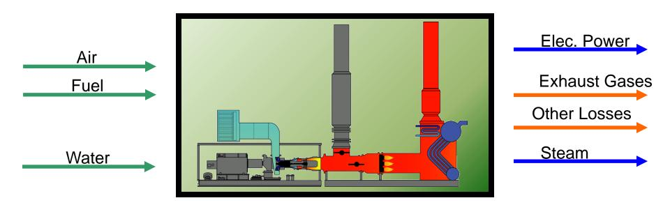
CHP Efficiency = Elec. Power + Steam Fuel Input
