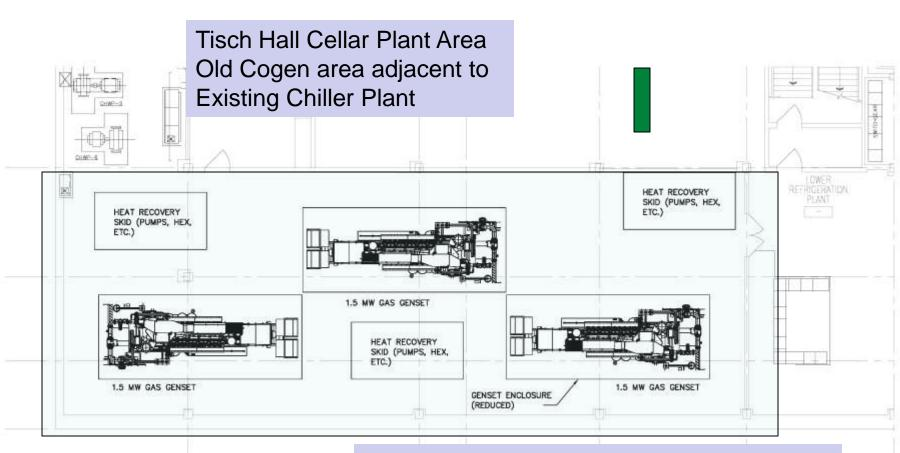
Tisch Electrical Proposed Alternate Scope Installation Scope Install 2 New Generators 3.2 MW (Nat Gas) Install 1 New Generator 1.6 MW (No 2 FO)
