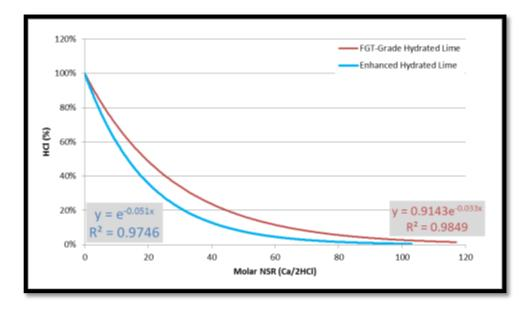
Gas temp = 540°F H2O in wet gas, % by wt. = 11.75% SO2-to-HCl ratio (lb/lb) = 92.6
