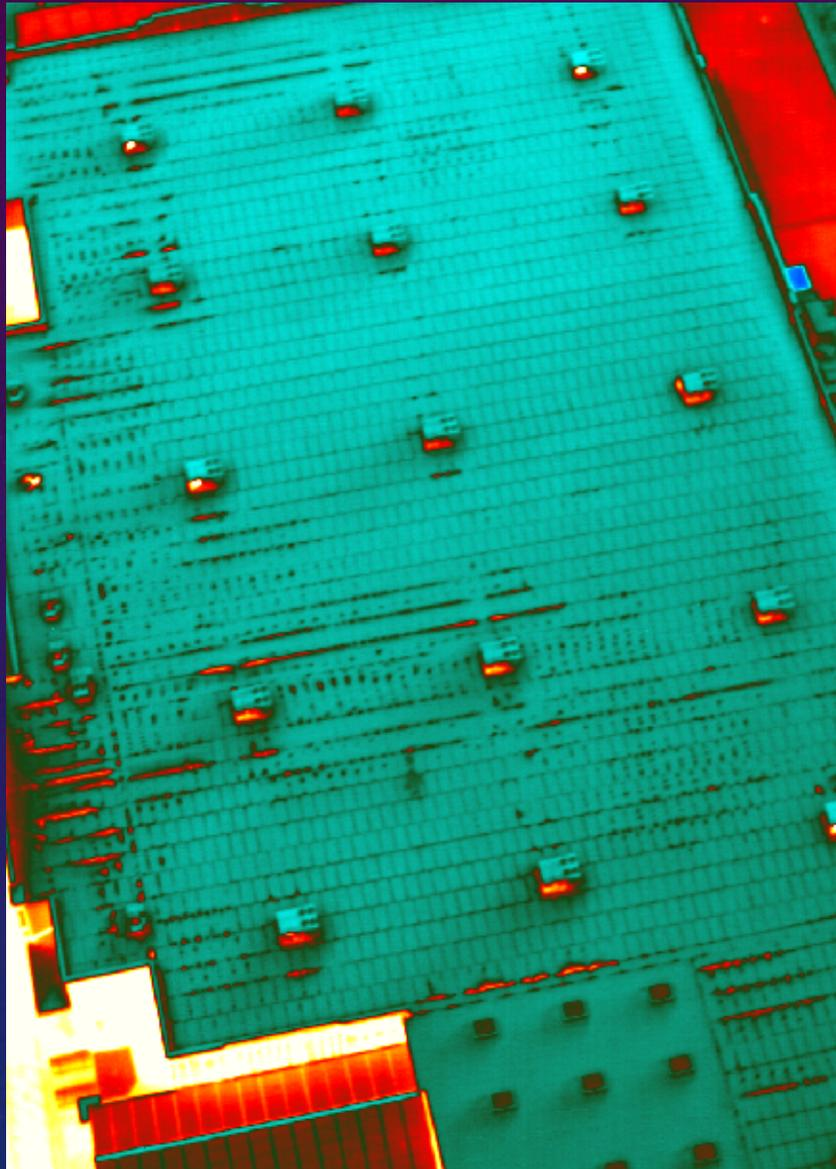
During the pressurization testing, ~50,000 CFM was supplied to the building with the procedure described in Reports 2. This raised the building pressure from normal (slightly negative) to .1 inches or ~25 Pascal).
