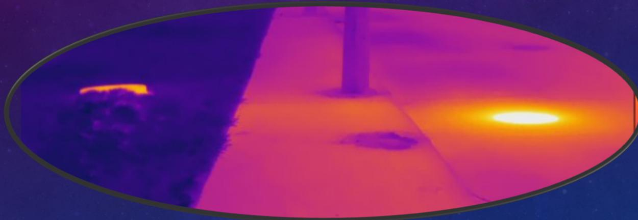
For example, five different apparent temperatures will result from the same temperature line that runs under a grass-covered field, an asphalt parking lot, a concrete loading dock, a gravel-covered area and a bare earth pathway.
