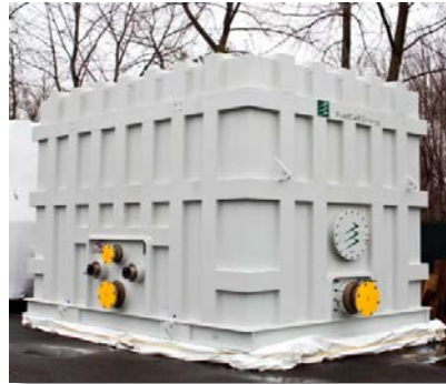
The stacks are enclosed, creating the fuel cell module
