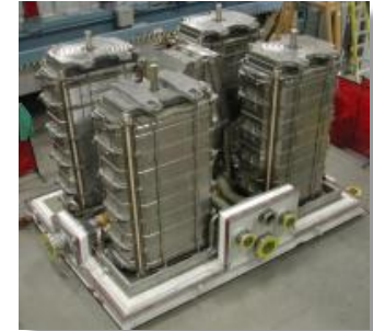
4 stacks are combined to build a 1.4 MW plant
