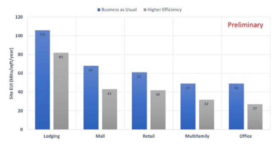
Example building energy simulation analysis to identify achievable energy use intensity values in different building types relative to business as usual; simulations were performed for DOE prototype buildings in the IECC 3a climate zone (Atlanta, Georgia) using OpenStudio/EnergyPlus workflows
