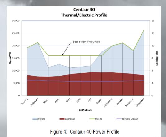
25,000 13 **Base Steam Production** 10 20,000 Hdd 15,000 8 10,000 - 5 5.000 - 3 W34 1. May October 2015 Month Steam Electrical — Steam ——Gas Turbine Output
