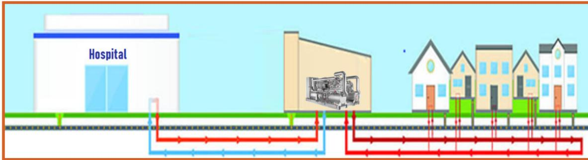
Simultaneously cooling the hospitals (1707 Tons, 5992 kW) and providing district heating (26614 MBH, 7800 kW) for other buildings
