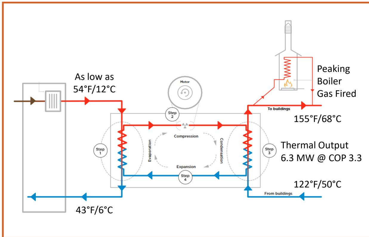
Fully packaged high temperature high lift centrifugal heat pumps will provide **155°F/68°C heating water** (21,500 MBH/6.3 MW) for connected buildings
