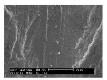
"Thumb-nail" shaped fatigue crack initiating at attachment weld on OD surface of tube.
