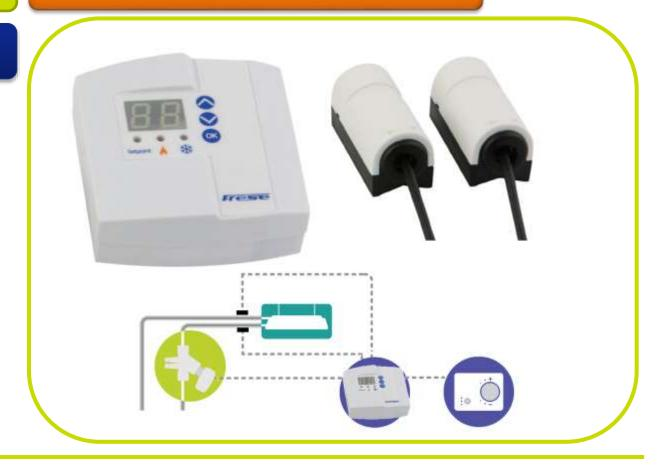
Frese Delta T is a supply and return temperature controller with two temperature sensors. Frese Delta T limits the flow through the terminal unit by means of a control valve in order to obtain the minimum required (designed) temperature difference in the supply and return lines of the system and thus enhance it's efficiency and optimize pump energy consumption.
