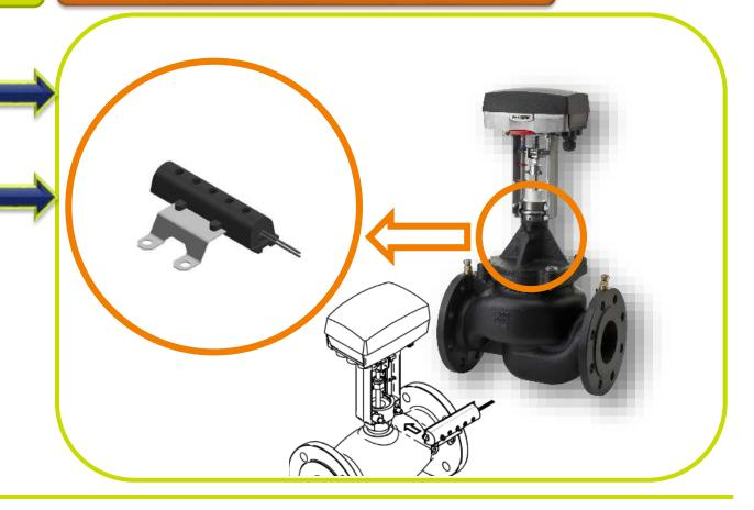
Frese Optima Compact DN40-200 can be offered with a stem heater. If sub zero media or low ambient temperature are expected in the system Frese Optima Compact must be provided with the stem heater. The stem heater uses 50W of heating power to prevent the ice building on the stem of the valve/actuator.
