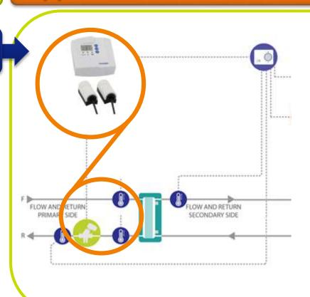
Frese DELTA T can be used in heat exchanging stations on the primary system side. Frese Delta T needs to be connected to the 2-way control valve (Optima Compact) that controls the temperature of water flowing on the secondary side of the system. By controlling the temperature difference between the supply and return line the optimized  $\Delta T$  is achieved, the pump pressure and flow in the district cooling system may be reduced and so the cost of running it.
