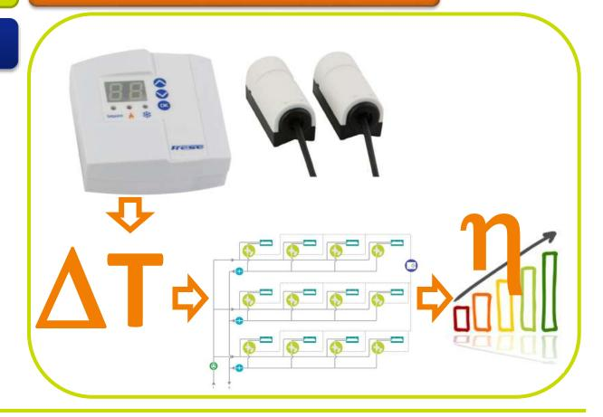
Frese Delta T makes that a hydronic system always operates with the possibly best efficiency. Even at partial loads when the flow to terminal units is much lower compared to sizing conditions Frese Delta T maintains the supply and return temperature difference on the required level. Consequently the flow can be just sufficient to secure the required capacity and at the same time the pump can run on low speed.
