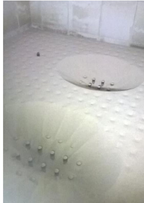
Primary air nozzles of the boiler become visible under the static sand bed during a sand removal test
