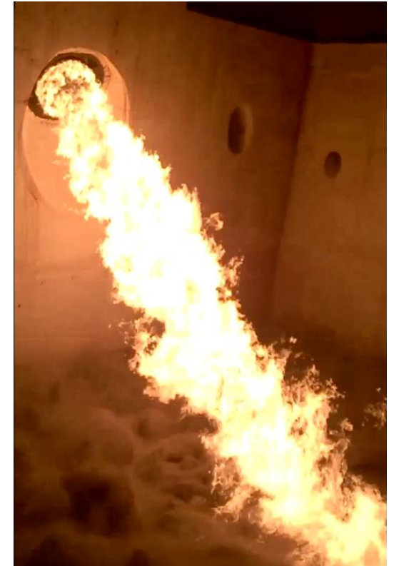
Heating the BFB sand bed with the start-burner to 350°C (660°F) before solid fuel feeding
