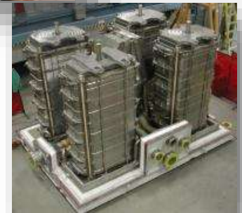
4 stacks are combined to build a 1.4 MW plant
