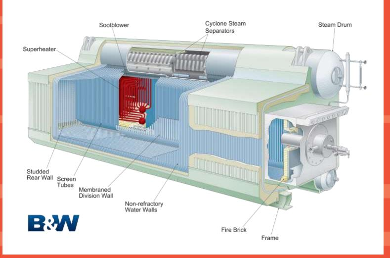
New 850 psig gas boilers provide best payback to feed 850 psig and 325 psig turbine generators.
