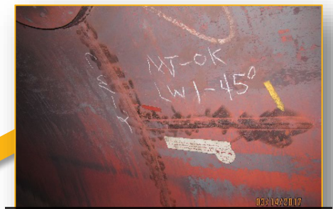
Critical welds tested - OK
