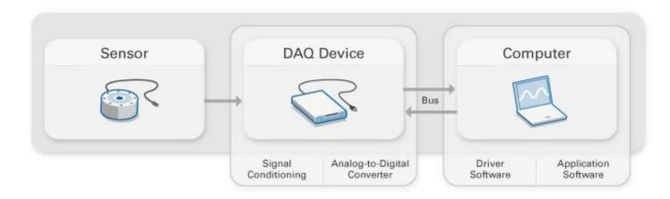
**Data acquisition (DAQ)** is the process of measuring an Thermal or physical phenomenon such as voltage, current, temperature, pressure, or sound with a computer. A DAQ system consists of sensors, DAQ measurement hardware, and a computer with programmable software.
