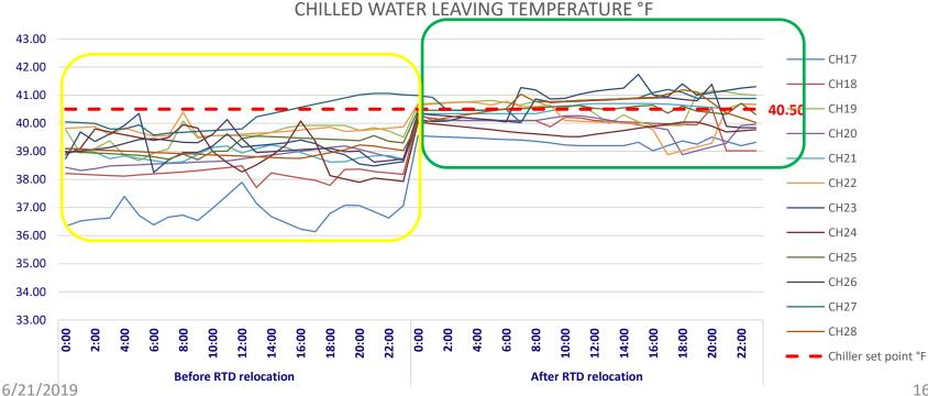
After the relocation of Chiller RTD of each chiller, the Chilled water leaving temperatures are close to the Set Point.
