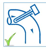
Install sensors against flow direction Install Sensors At the correct angle.
