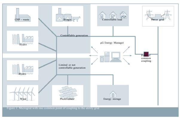
According to this definition, a microgrid maximizes the benefits of distributed generators and solves the above-mentioned disadvantage, also utilizing distributed generation during utility power system outages.
