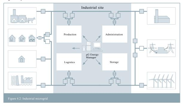
Typical examples are chip manufacturing, the chemical industry, and the paper and foodstuff industries, for instance. Today, some industrial sites are installing uninterruptable power supplies if their utilization is economically justified. Microgrid structures may bring additional advantages, for example the combination of secure power supply with high energy efficiency and the utilization of renewable generation.
