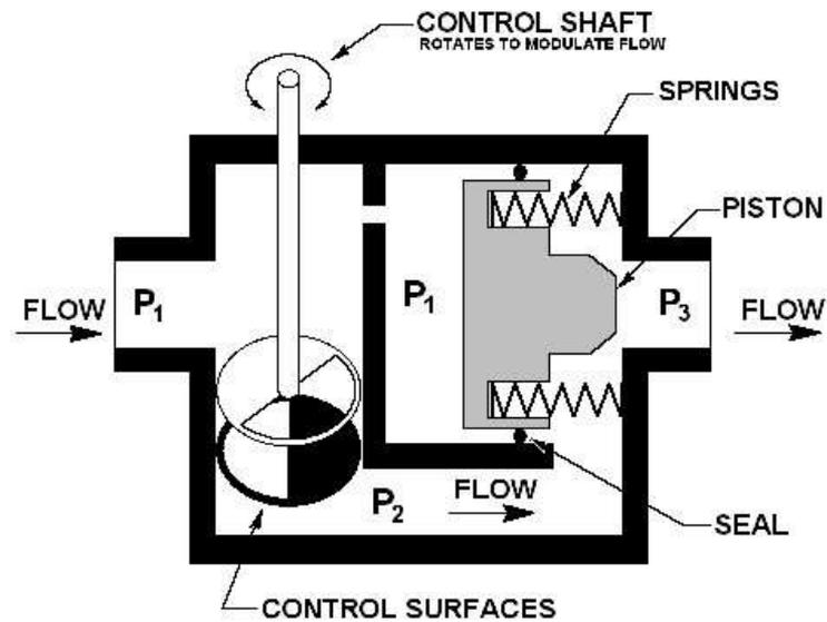
Flow is steadied by maintaining constant differential pressure across the control surface
