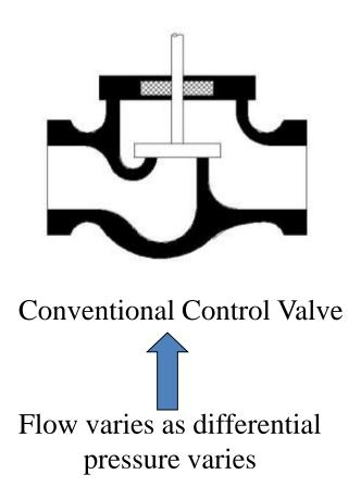
Conventional control valves must react to both load and pressure changes
