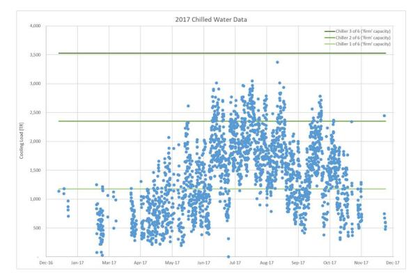
Air Conditioning, Peak ~3500Tons, 42-degree Chilled Water
