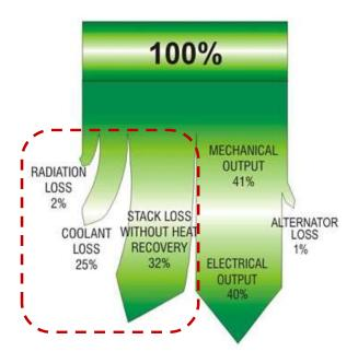
Overall System Efficiency with Heat Recovery = **75 - 80 %** 100% Heat Recovery - HT Jacket Water waste heat 18% + Exhaust Flue gas 22% STACK RECOVER 22% MECHANICAL RADIATION LOSS 2% 41% ALTERNATOR COOLANT LOSS 1% 7% ELECTRICAL OUTPUT 40% STACK LOSS AFTER HEAT RECOVERY POWER + PROCESS HEAT & COOLING 10% 80%
