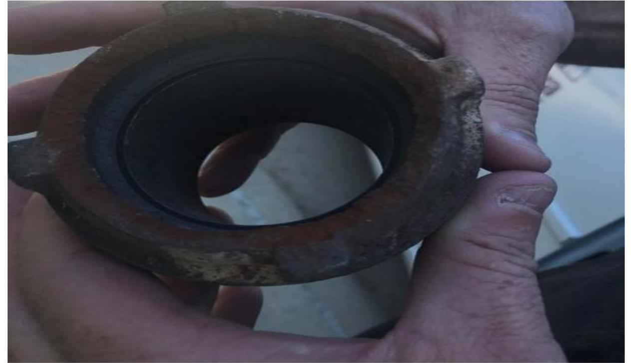
Figure 3: The failed cap after it had been removed from the steam pipe.
