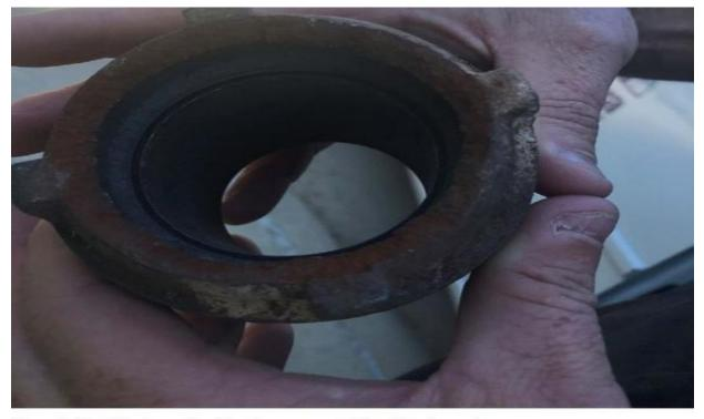
Figure 3: The failed cap after it had been removed from the steam pipe.
