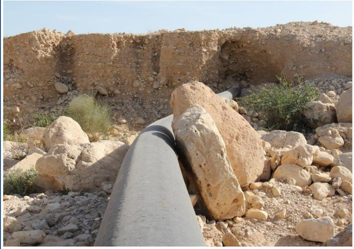
NO Slow Crack Growth: A 16" PE-Xa pipe installed in 1999, under constant load on an bedded ground.
