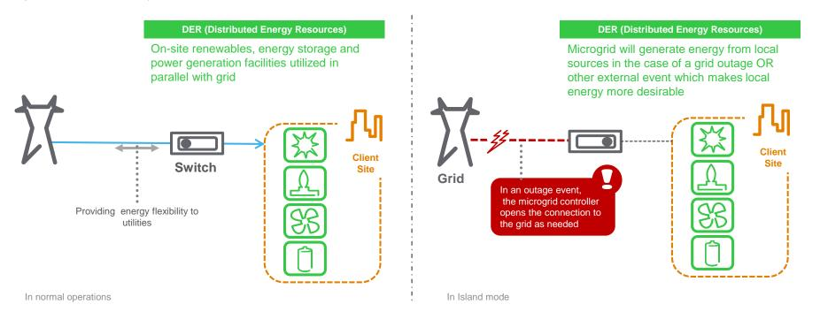
...which as an integrated system can operate in parallel with the grid or in an intentional islanded mode.
