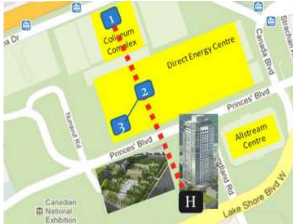
Figure shows new low-carbon thermal energy network (district energy) interconnecting 3 existing energy plants and supplying energy to new Hotel.
