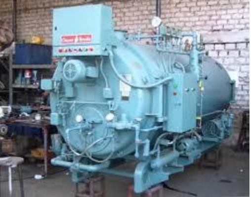
Gas “package” boiler: water in, steam out
