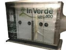
CHP packaged at factory, some site assembly
