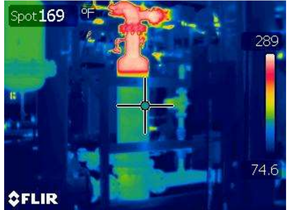
Heat Map Showing Tube Flooding to Avoid Flash
