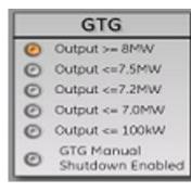
If the GTG output drops below 7.2 MW -initiates automatic staggered opening of the Lot 25 PV output stages (108 kW/stage). The first Lot 25 PV stage will immediately open, and every 10 seconds later another stage will automatically open until all stages are opened, or the GTG output increases above 7.2 MW.
