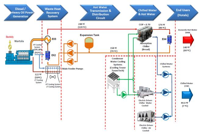
This system provides 5,000 RT of chilled water and domestic hot water (DHW) to hotels located near to CEMP's power plant. Waste heat comes from the exhaust gases and cooling water of diesel engines (6 MWe each) that consume heavy fuel oil (HFO).
