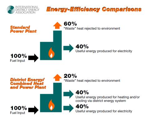
From the data of International District Energy Association (IDEA), It is easy to know that the energy efficiency of a standard power plant is only 40%, and that of 60% is wasted as the waste. However, with the same fuel input, the energy efficiency can be 80% if the power plant combined heat and cooling. Obviously it will benefit a lot not only in saving energy cost but also to the environmental protection.
