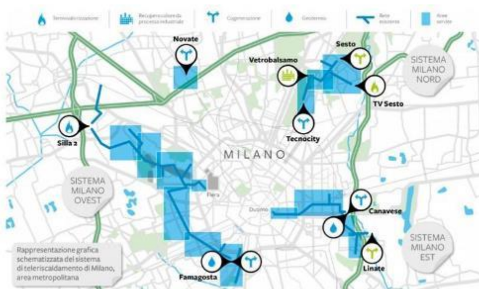
Pic. Milan's district heating system representation. In the image the three current networks, the different plants and service areas can be seeing. A2A district heating Design for Sustainability, 2017.
