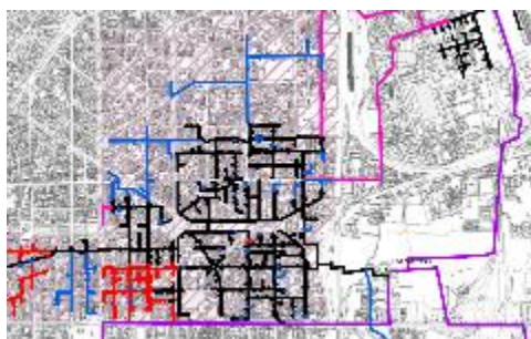
Pic. A portion of Milan's district heating network, connected to the Canavese CHP plant. Milan's segregated networks are undergoing interconnection and expansion to form three large heat networks by 2016, which will then be interconnected via a ring around the city.
