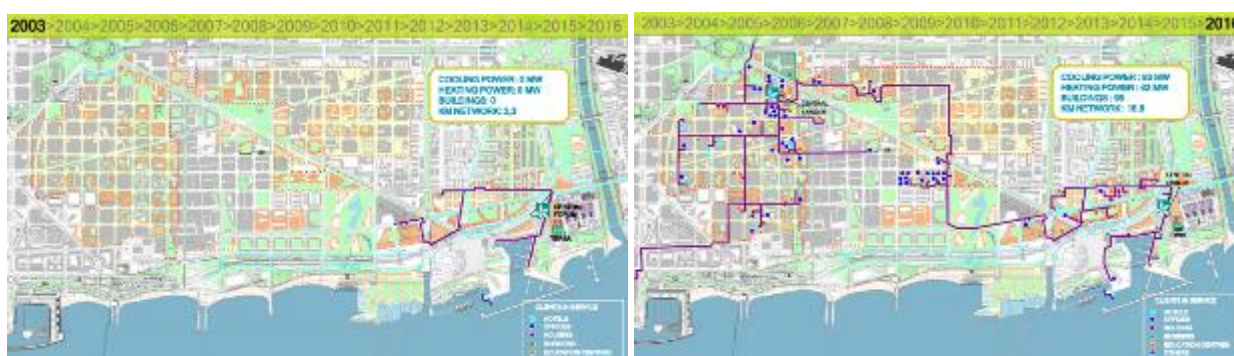
Pic. From 2003 to 2016 cooling power from 0 MW increased to 93 MW, heating power from 0 MW to 62 MW respectively. District Heating Network from 3,3 km increased to 16,8 km.
