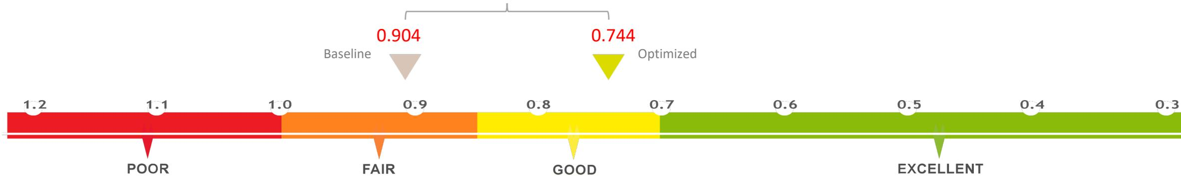
Average annual chilled water plant efficiency in kW/ton.
