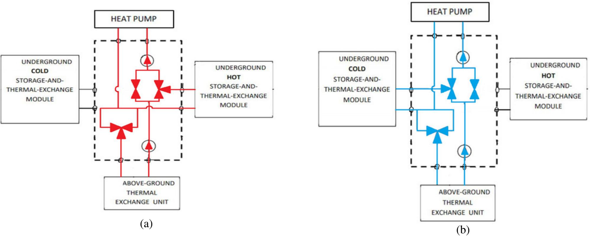
Parallel modes using (a) hot module and (b) cold module [4]
