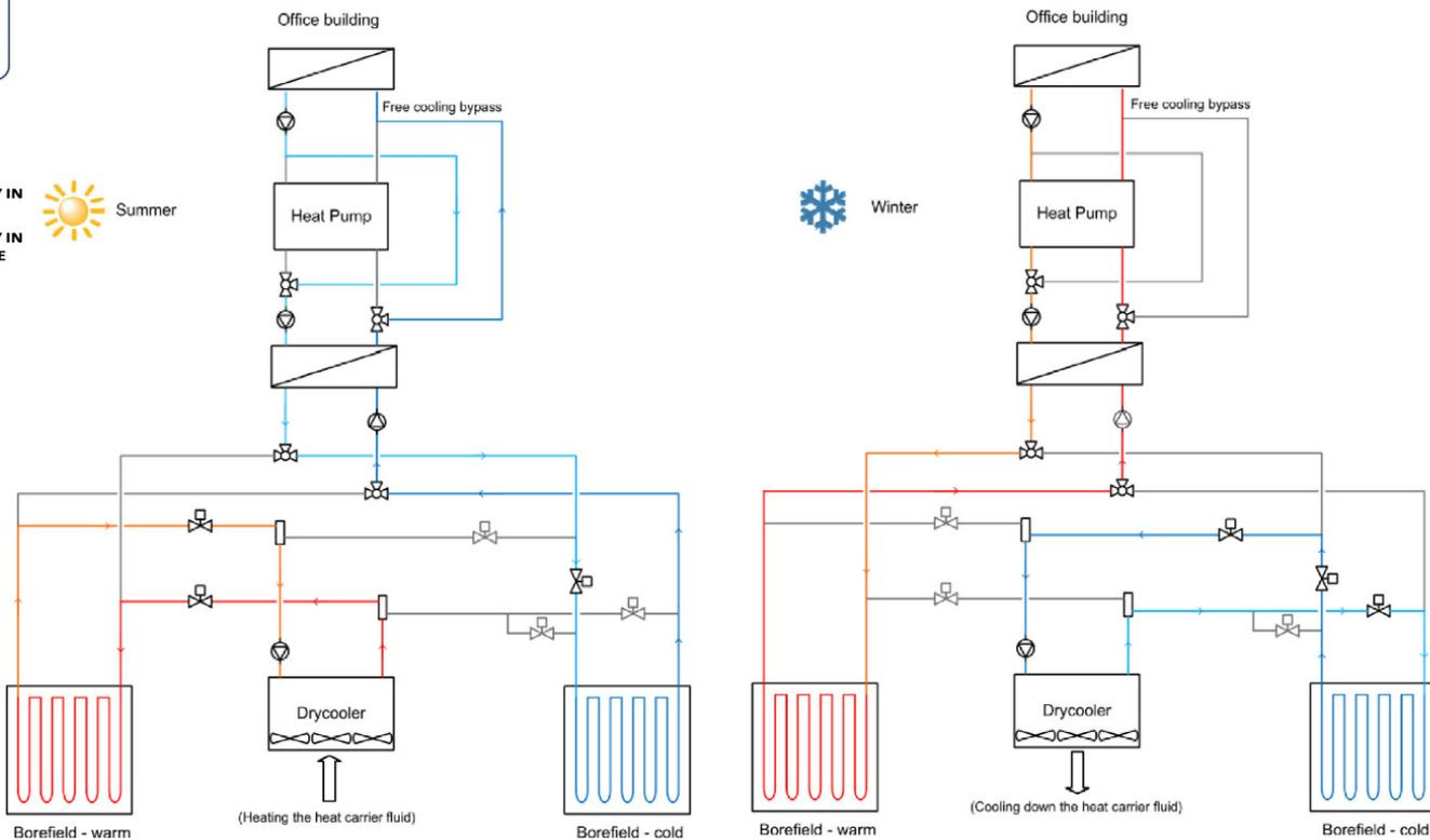
Multi-source system design: (a) cooling mode (b) heating mode [1]
