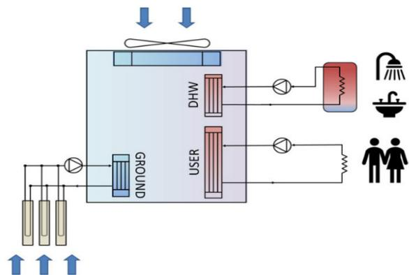
Dual source heat pump system design [2]
