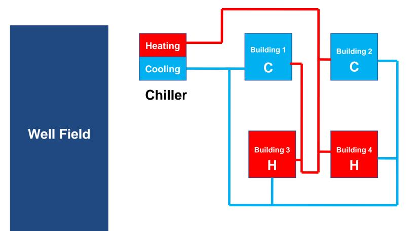
Simultaneous Heating/Cooling COP > 7
