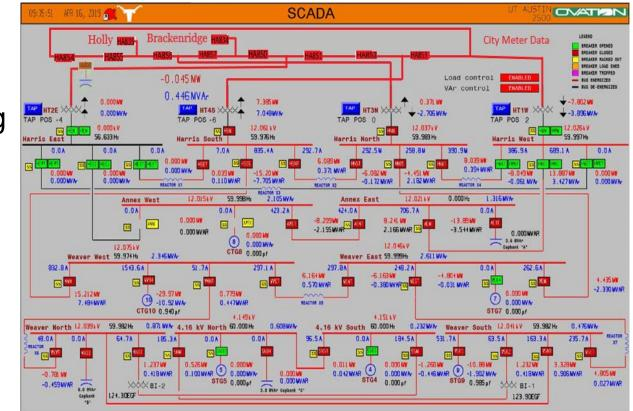
UT Microgrid has all main control functions encountered in other typical installations:
