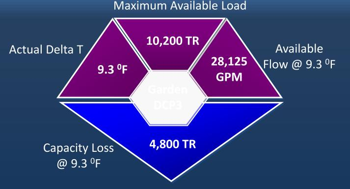
It is confirmed from the operation data that plant was not producing design tonnage with a huge capacity loss because of low delta T.
