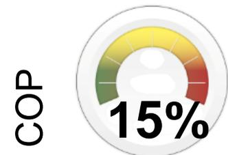
**A reduction of return temperature of chilled water can lead to a 15% drop of the COP**
