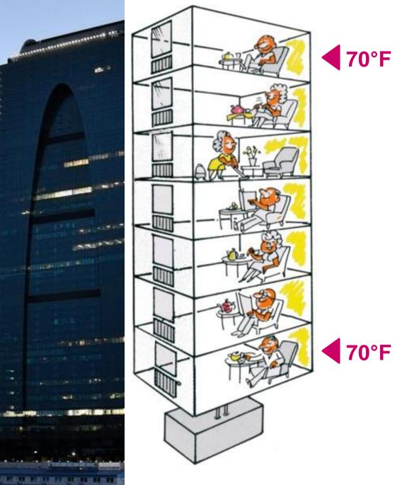
With hydronic balancing, all circuits gets design flow at the same time.
