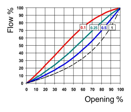
ASHRAE Handbook 2016 HVAC Systems and Equipment, Ch 47 (Valves) The selection of the control valve pressure drop directly affects the valve authority and should be at least 25 to 50% of the system loop pressure drop (i.e., the pressure drop from the pump discharge flange, supply main, supply riser, supply branch, heat transfer coil, return branch, fittings, balancing valve, and return main to the pump suction flange).
