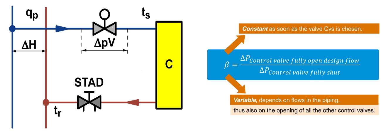
In a *variable* flow distribution, the authority of a control valve is *variable*.
