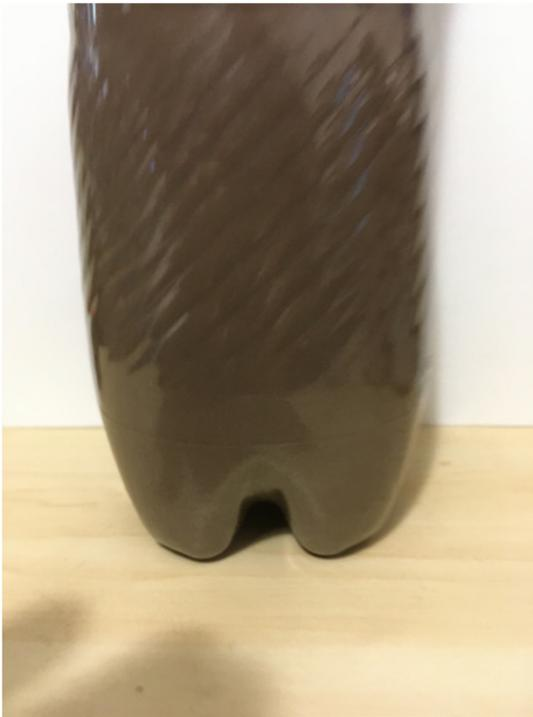
**Current Separators limited Removal -Settling after 3 Minutes**
