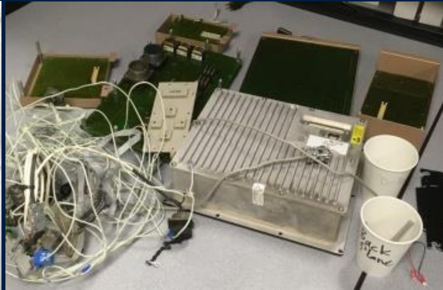
Custom-built electronics removed from TQG
