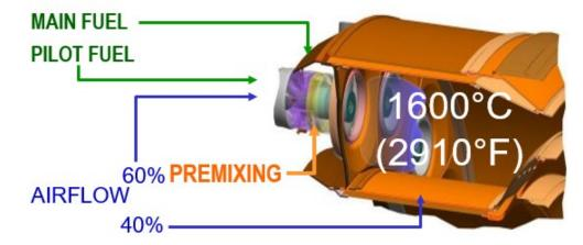
Gas Turbine SoLoNOx Combustion
