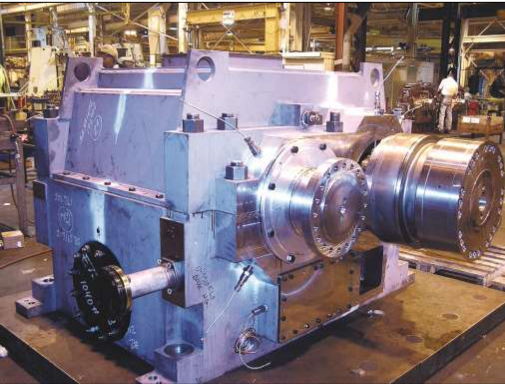
Clutch quill-shaft mounted with internal bearing
