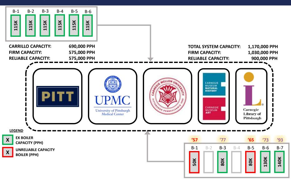
BELLEFIELD CAPACITY: 480,000 PPH FIRM CAPACITY: 340,000 PPH RELIABLE CAPACITY: 210,000 PPH
