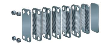
Plate geometry cause flow to whirl, Flow is turbulent already at Re 150 Self-containing structure >95% of material used for heat transfer
