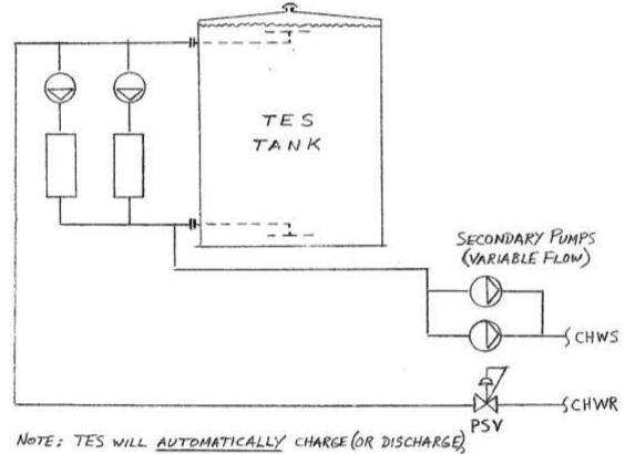
BASED ON PRIMARY FLOW BEING MORE (OR LESS) THAN SECONDARY FLOW.
