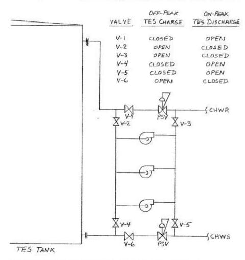
PSV = PRESSURE SUSTAINING VALVE (BACK-PRESSURE CONTROL VALUE)
